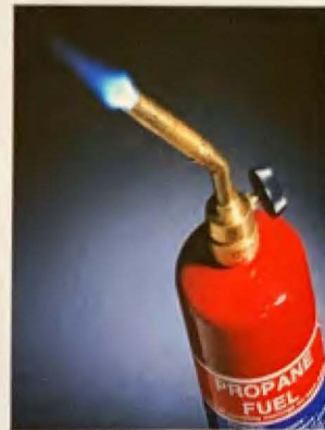
\blacktriangleright Figure 3.8 Propane burning in air. Liquid propane in the tank, C_3H_8 , vaporizes and mixes with air as it escapes through the nozzle. The combustion reaction of C_3H_8 and O_2 produces a blue flame.
